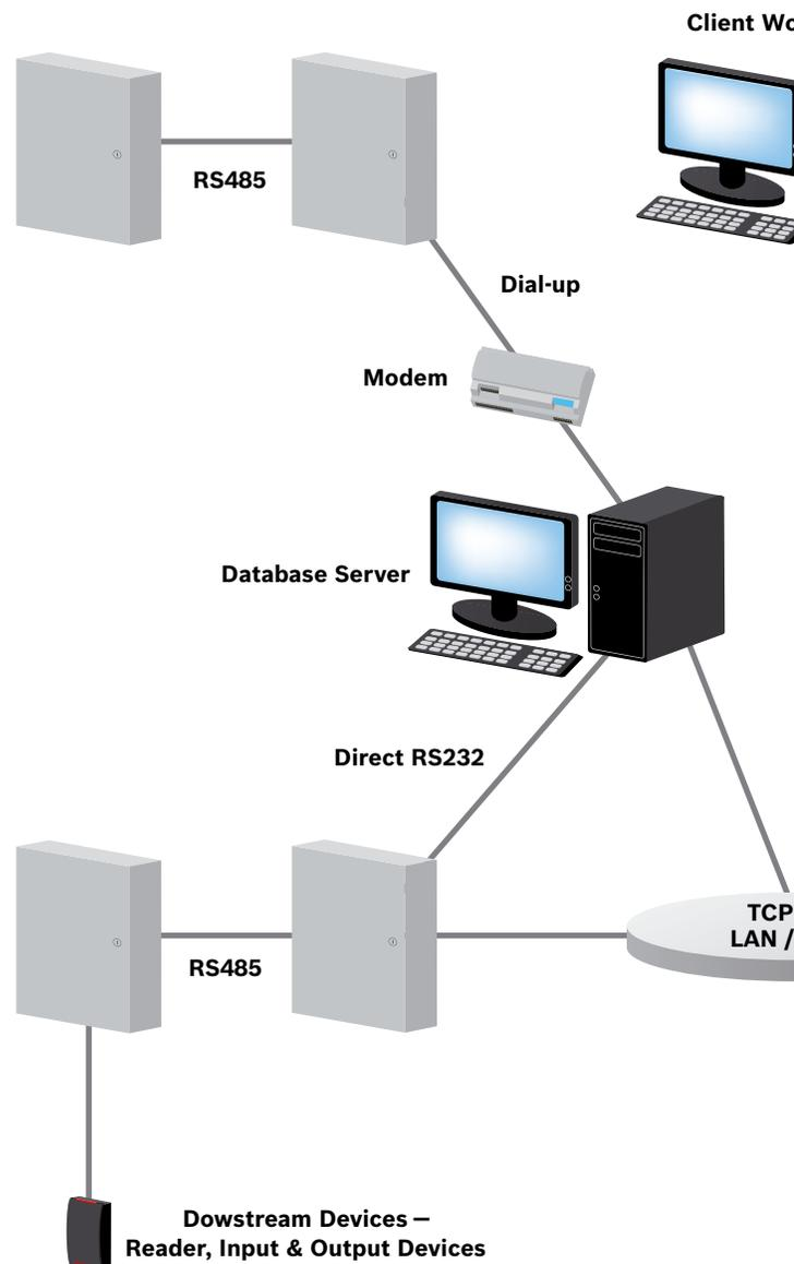
The system links gracefully with existing Bosch G Series security control panels, the Conettix D6600 Receiver/Gateway, CCTV equipment, and even devices from other manufacturers – including biometrics fingerprint readers.
